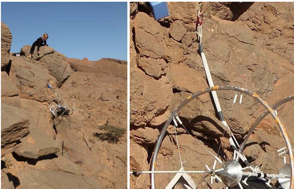
*Vehicle blockage at the end of test 96: the anti yaw rod is engaged (and slightly bent) between two blocks. Under the vehicle (left photo) the black pole which will be used to push it upwards is visible.*
