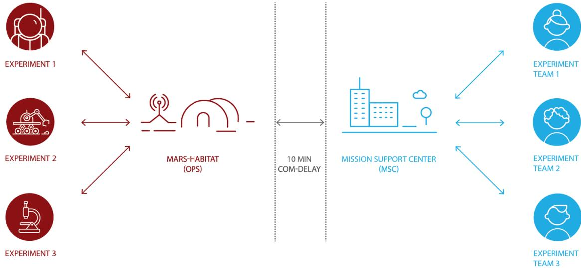
Conceptual architecture of the AMADEE-24 expedition: A 10min time delay reflects the signal travel time between Earth and Mars. The MSC in Innsbruck/Austria was the single-line-of-contact between “Earth” and “Mars”.
