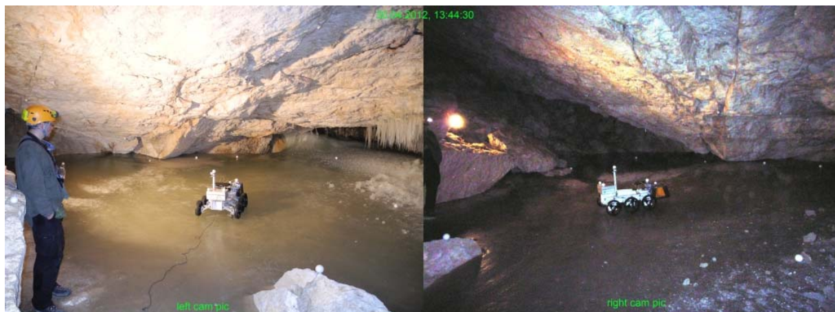
Figure 2: External tracking of the WISDOM unit by a stereo camera setup
